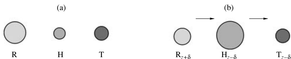
Fig. 7. Changes in atomic radii in going from (a) \text{ErNi}_3\text{H}_{4.0} (small lattice anisotropy) to (b) \text{CeCo}_3\text{H}_{4.0} (large anisotropy).
