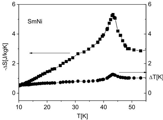
**Fig. 5.** Left side: (○) magnetic entropy change,  $\Delta S_M$ , estimated from heat capacity measurements as a function of temperature in the range of 2–55 K for  $\Delta H = 5$  T. Right side: (●) adiabatic temperature change,  $\Delta T_{ad}$ , as a function of temperature calculated from heat capacity measurements.
