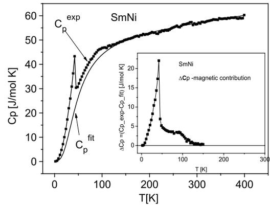
**Fig. 6.** The results of heat capacity measurements on SmNi in the 2–400 K temperature range. The full line represents the lattice specific heat contribution calculated for a number  $N_D = 6$  of Debye-like modes with an average Debye temperature  $\theta_D = 199$  K. In the inset, the magnetic contribution of  $\text{Sm}^{3+}$  ion magnetic moments to  $C_p(T)$  for SmNi is displayed.
