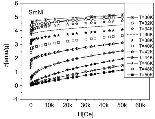
**Fig. 2.** Magnetization curves versus magnetic field for several temperatures around  $T = 42$  K.
