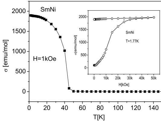
**Fig. 1.** Temperature dependence of the magnetization ( $\sigma$ - $T$ ) of a polycrystalline SmNi sample measured in the 2–150 K temperature range in the field cooling procedure (FC). The inset shows the ( $\sigma$ - $H$ ) curves at 1.77 K up to 5 T.
