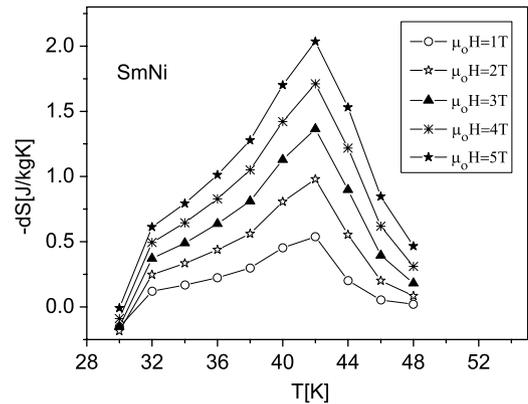
**Fig. 3.** Temperature dependence of magnetic entropy changes in SmNi for field changes of 1, 2, 3, 4 and 5 T.
