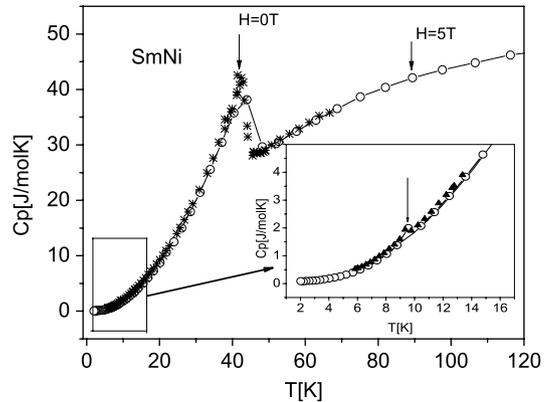
**Fig. 4.** Heat capacity of SmNi versus temperature in zero and 5 T magnetic fields in the 2–150 K temperature range. In the inset, the details for  $C_p(T)$  measured around  $T = 10$  K are presented. Open circles (O) and the full line display the  $C_p(T)$  data in zero and 5 T, respectively, registered with the PPMS. The full triangles (▲) show  $C_p(T)$  data taken in zero magnetic field using the homemade apparatus.
