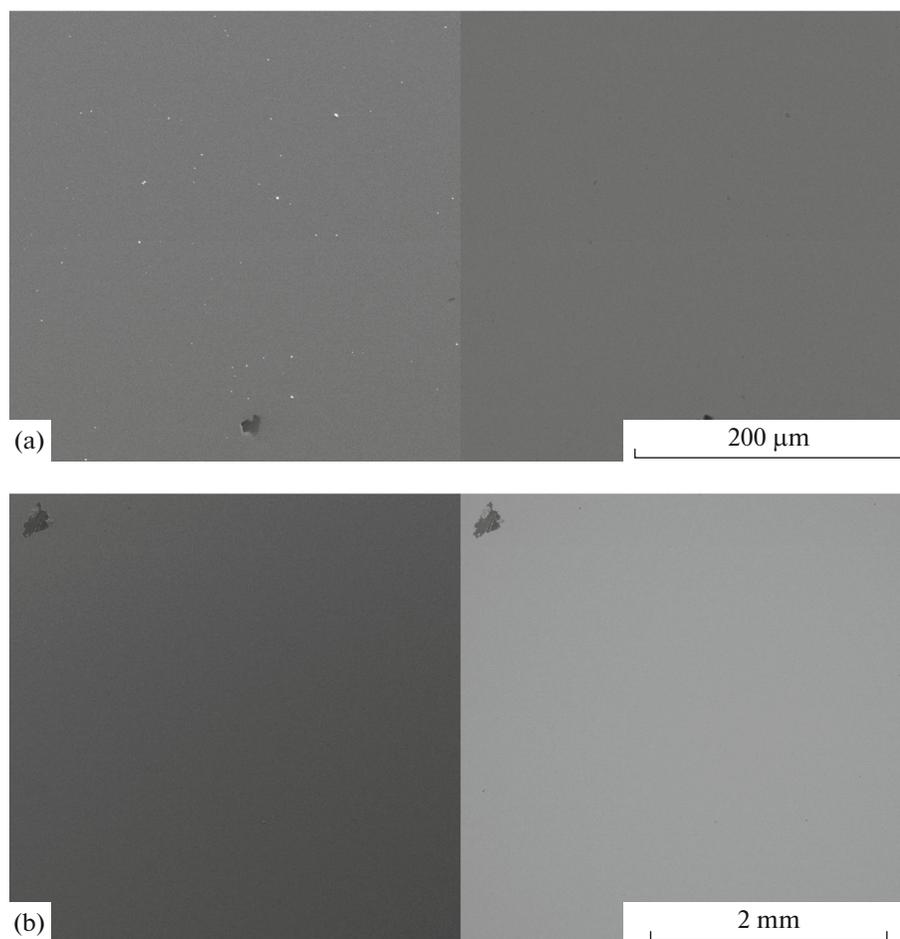
**Fig. 1.** SEM micrographs of films of metals deposited on the surfaces of silicon substrates: (a) cerium (chromium protective layer); (b) cerium (nickel protective layer). Images are presented in the mode of secondary electrons and backscattered electrons.
